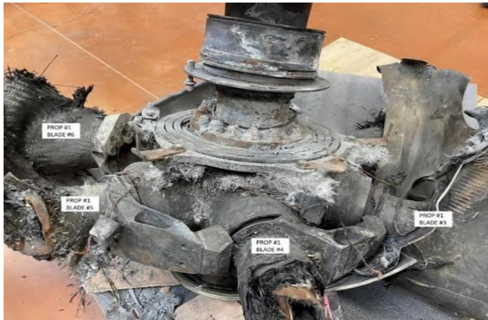
Figure 25 Prop #1 hub assembly
