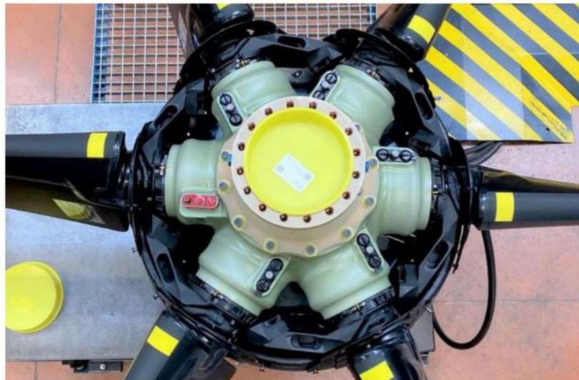
Figure 21 OEM propeller on Ratier-Figeac assembly line displayed in Feather position
