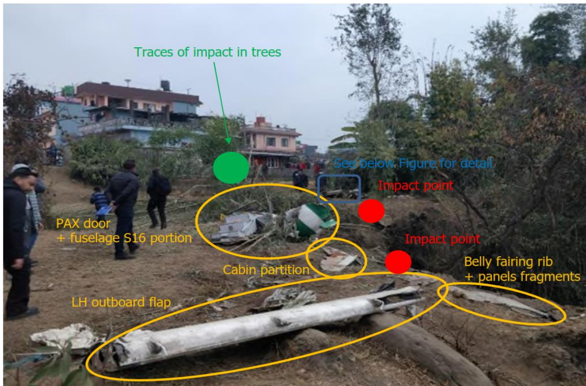
Figure 13 Site A- Identified impact points and parts
